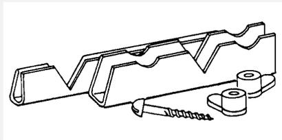
EASYFIX double glazing pre-packs are an alternative to the loose packed items mentioned so far. A 15m or 30m kit in any of the edging strip sizes or colours, comes complete with sufficient clips, screws and a mitre gauge to fix the edging strip provided. Full fitting instructions are included in the pre-pack.
