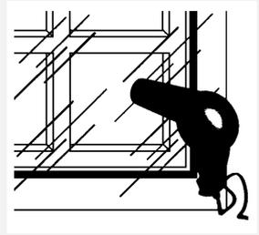
FILMGLAZE can be used on individual windows, or over the complete window area. Handles and locks can be removed and replaced after the film has been applied. Being a simple film it allows for quick access in cases of emergency.
