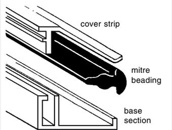
**HELPFUL HINTS** - To achieve a neat mitre cut a small piece of mitre bead and insert between the base and cover strip at the point where the mitre is to be cut. Cut the mitre through all sections. This beading has the effect of holding the cover strip at the correct angle so that when applied to the sheet it results in a neat mitre.
